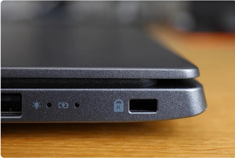
Figure 3.4 A standard security slot on a thin laptop. Check yours against the model's manual before buying a lock.
