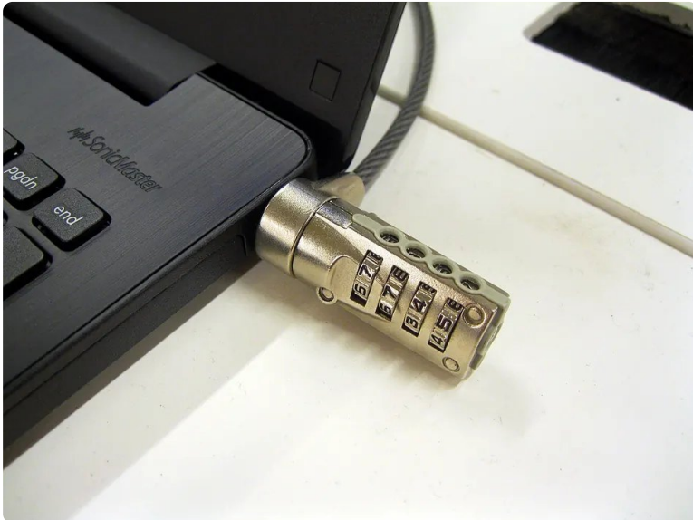
Figure 3.2 A combination cable lock in use. The loop around a fixed object matters as much as the head in the slot.
